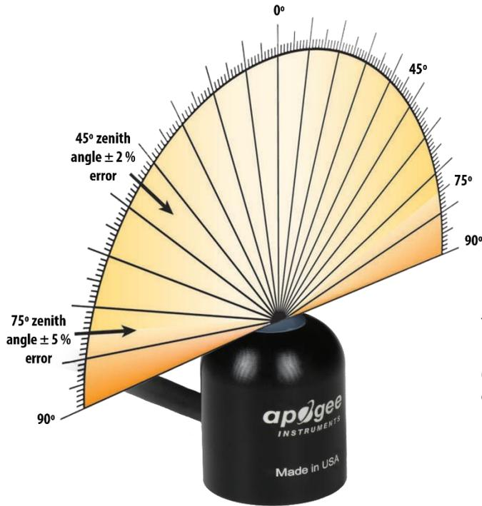
Directional, or cosine, response is defined as the measurement error at a specific angle of radiation incidence. Error for Apogee SQ series quantum sensors is approximately ± 2 % and ± 5 % at solar zenith angles of 45° and 75°, respectively.
